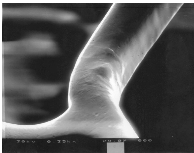
Figure 7. SEM micrograph of a dilated S-shaped region with high mechanical stress (magnification: 350).
