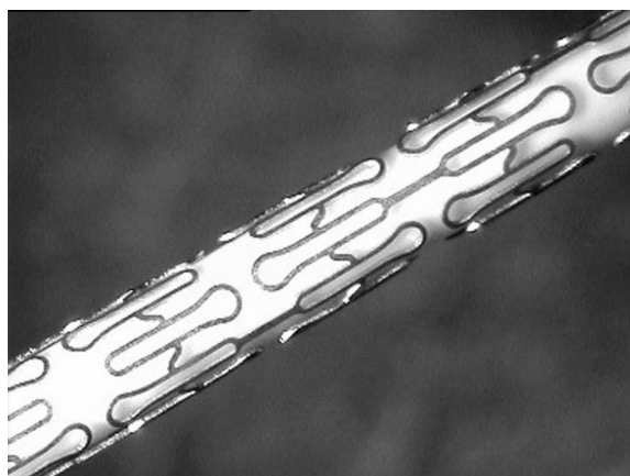
Figure 3. TENAX preform after laser cutting and pickle treatment using an ultrasonic cleaning equipment.
