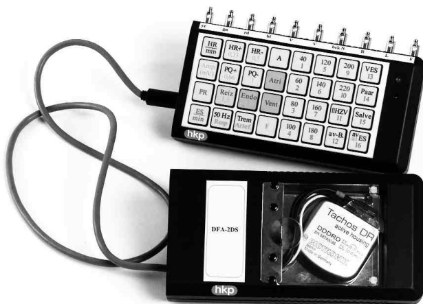
Figure 1. Arrhythmia Simulator (ARSI, HKP, Germany). The device consists of the simulator itself (top) and the ICD adapter (DFA - 2DS, bottom). Pressing the <PR> button and any of the numbers on the simulator will start a group of tachyarrhythmias, e.g., AV nodal reentrant tachycardias with varying VA interval. Single or multiple atrial or ventricular extrasystoles may be delivered by pressing one of the 4 buttons at the far right of the panel. Even noise generated by alternating current or skeletal muscle can be generated. The adapter accommodates the ICD through the pocket created during device implantation, and even facilitates testing of an active can device. The ICD is attached via standard DF-1 connectors, mimicking the defibrillation electrodes, and IS-1 connectors for the pacing and sensing leads.
