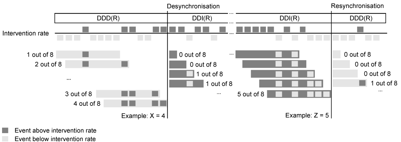
Figure 3. Automatic mode switching in the dual-chamber pacemakers Philos DR, D, and SLR: Schematic depiction of the functioning of the X/Z-out-of-8 algorithm, with the switch-on criterion X set to 4, and the switch-off criterion Z, to 5.
