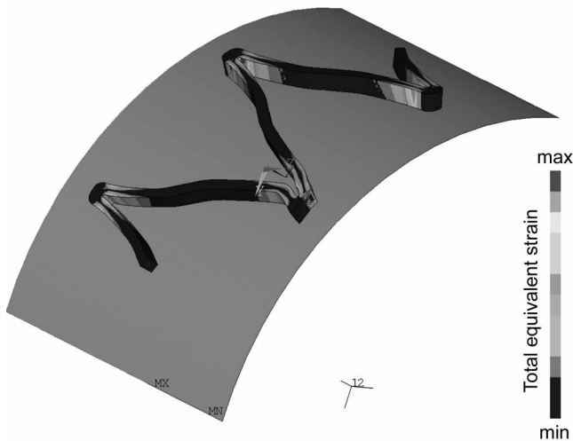
Figure 16. Depiction of equivalent strain as per v. Mises after the expansion of a stent segment.
