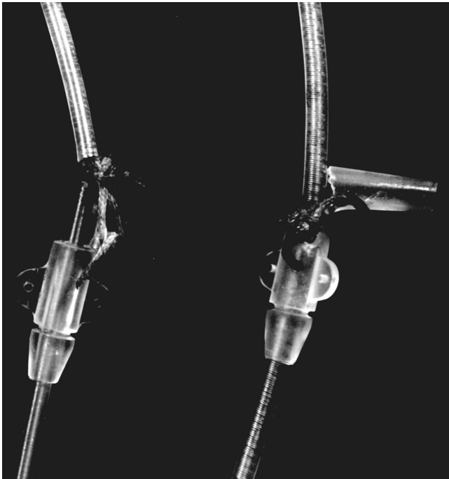
Figure 3. Two lead bodies and the sleeves with the suture remnants are represented in detail. At the lower part, the atrial lead is presented with the torn sleeve. The insulation of the body was slightly constricted (not visible). At the upper part of the figure, the ventricular lead body and the cut sleeve can be seen. Not only the outer insulation and the outer (proximal) coil are disconnected, but also the insulation around the inner (distal) coil, which explains the total loss of sensing and pacing.
