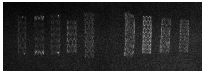
Figure 9. X-Ray picture of expanded coronary stents - From left to right: Sorin Carbostent; Biotronik Tenax XR; Medtronic beStent Brava; Cordis Bx Velocity; Cordis Crossflex; Scimed NIR Royal; Medtronic AVE S670; ACS RX Multilink Tristar.
