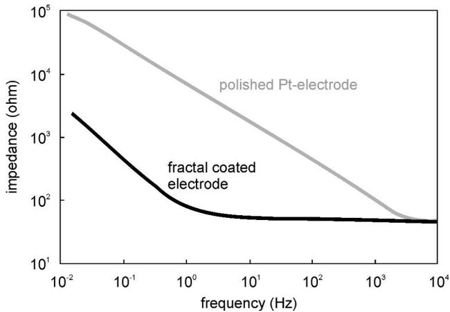
Figure 1. Charge transfer impedance of a polished platinum electrode (gray line) and the fractal coated iridium electrode (black line).
