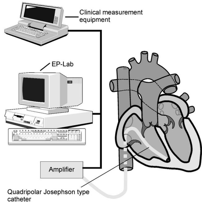
Figure 2. Clinical equipment for monophasic action potential measurements in our study.
