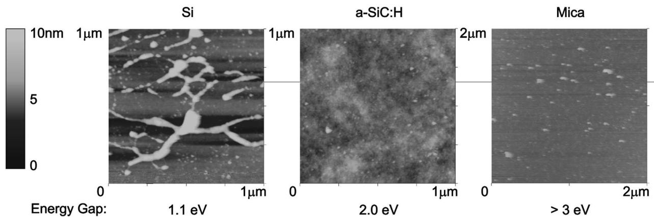
Figure 5. Scanning force microscopy-images done in the "tapping mode" of Si-, a-SiC:H- and mica-surfaces incubated with fibrinogen solution (6 μg/ml). The energy gaps of the materials are 1.1eV (Si), 2.0eV (a-SiC:H) and >3eV (mica).
