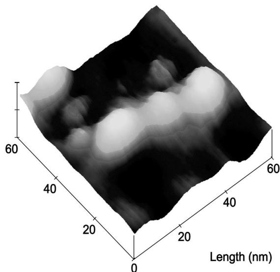
Figure 1. Isolated fibrinogen molecule imaged by AFM in the "tapping mode" on silicon (1 µg/ml fibrinogen).
