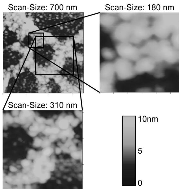
Figure 3. Fibrin network imaged by AFM in the "tapping mode" on silicon ( $4 \mu\text{g/ml}$  fibrinogen). In the two sections, single fibrin molecules are clearly resolved.
