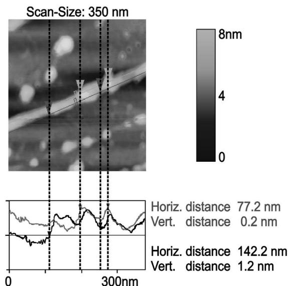
Figure 4. Fibrin strand imaged by AFM in the "tapping mode" on silicon ( $4 \mu\text{g/ml}$  fibrinogen). The two adjacent profiles show the displacement of neighboring fibrin molecules.
