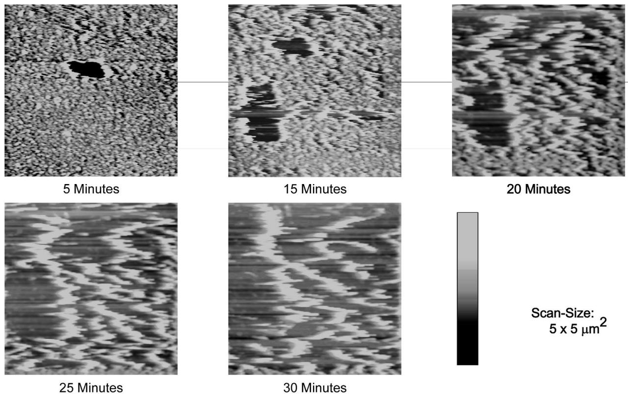
Figure 6. Development of fibrin strands imaged at the silicon-solution phase boundary by AFM in the "contact mode". Physiologic saline solution with 6 μg/ml fibrinogen.
