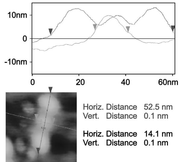
Figure 2. Isolated fibrinogen molecule imaged by AFM in the "tapping mode" on silicon (1 µg/ml fibrinogen) with the corresponding profiles of the protein.
