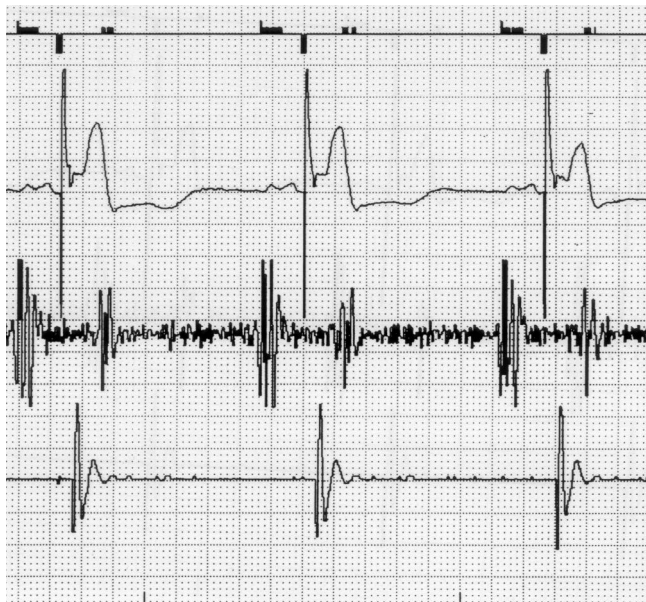
Figure 1. Presence of an atrial refractory sensed event on the marker channel (top of the figure) following the ventricular marker and corresponding to FFRS. The FFRS time reaches here 110 ms. From top to bottom: marker channel, VII ECG lead, atrial filtered electrogram, ventricular filtered electrogram.
