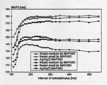
**Figure 4.** Electrical restitution curve (ERC) at 600 ms compared for Ag/AgCl-electrode, small tip electrode, and medium tip electrode.
