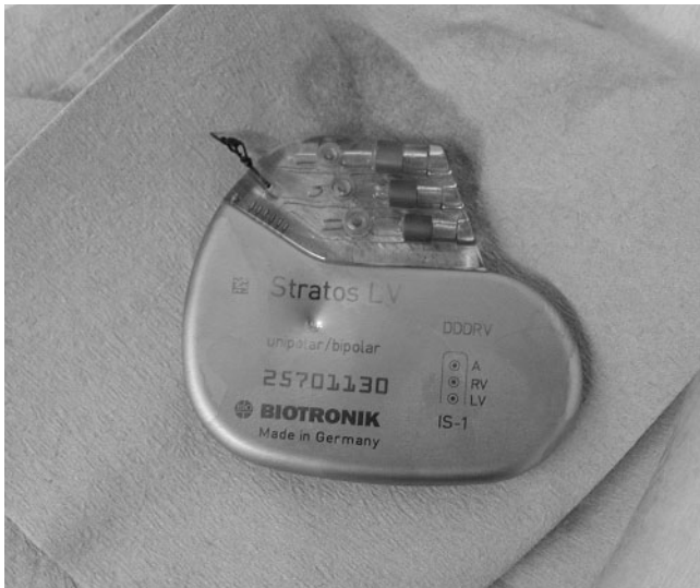
Figure 2. Chewed pacemaker. Faulty interrogation required replacement of this device.
