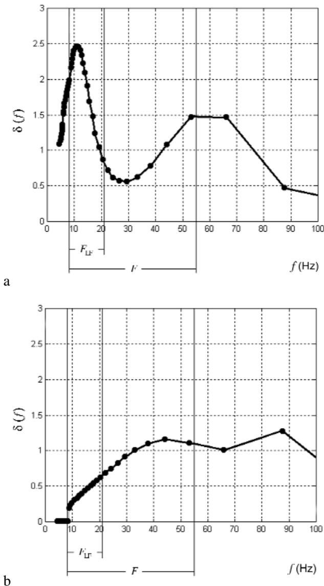
Figure 1. Frequency dependence of the transmission coefficient  $\delta(f)$  for the wavelet components of the atrial monophasic action potential (MAP) signals measured in the same patient, but in two different cardiac cycles. The resonance quality factor (see text) has considerably different values for the two beats:  $R = 44.9\%$  (panel a) and  $R = 18.7\%$  (panel b). Here  $F$  is the band used for the analysis and  $F_{LF}$  is the low-frequency band.
