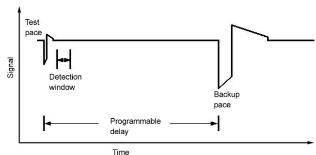
Figure 3. Test pulse sequence.
