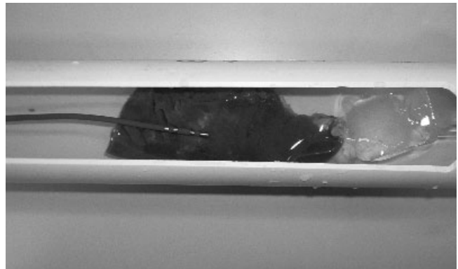
Figure 1. Panel a) Catheter and container; Panel b) amplified catheter tip, ice, and cow's heart.
