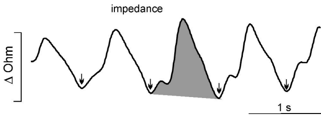
Figure 1. Calculation of the area under the Z curves using minima and maxima as boundaries.
