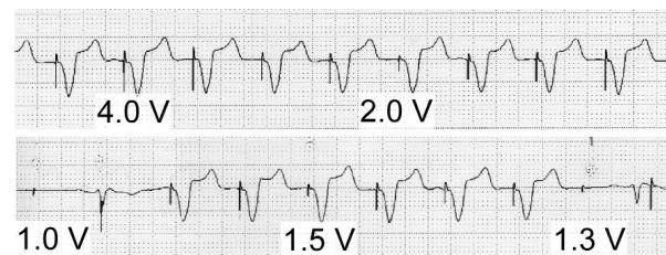
Figure 2. ECG recording of the automatic testing algorithm. The pulse amplitude is decreased every fourth beat by the half, if capture is detected. The three beats in between are at save value (4 V).
