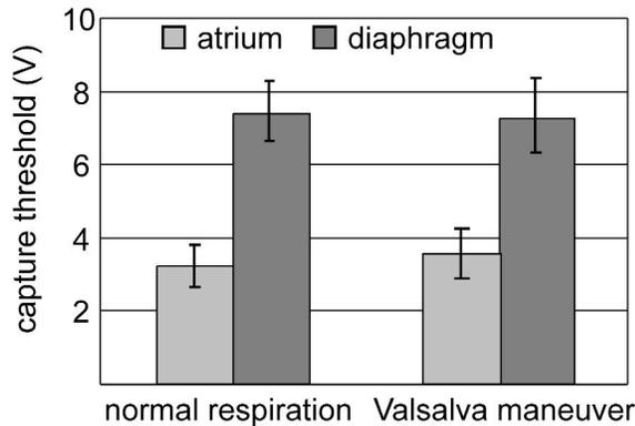
Figure 6. Atrial and diaphragmatic capture threshold with normal respiration and Valsalva maneuver (pulse width: 0.5 ms; n = 10).
