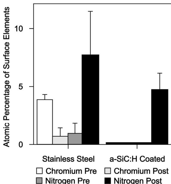
Figure 6. Chromium, used as a marker for stainless steel was found before circulation to almost 4%, whereas a-SiC:H completely covered chromium. After circulation the exposed chromium concentration was reduced to 0.7% and replaced by an increased nitrogen concentration, representing protein deposition. On a-SiC:H also nitrogen was deposited, though to a lesser extent.
