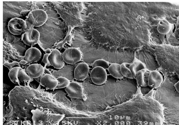
Figure 4. (a) Scanning electron micrograph (1500x) of the stainless steel surface showing areas with a dense layer of blood proteins and formed elements, covered by fibrin strands; (b) Scanning electron micrograph (2000x) of the a-SiC:H coated surface showing areas with thrombi and erythrocytes, but not densely packed and not extensively covered with fibrin.
