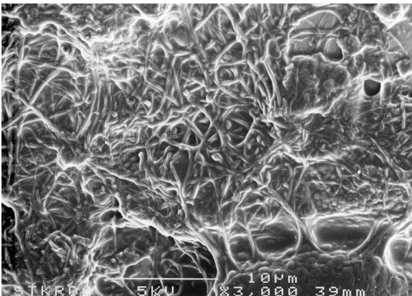
Figure 5. Detailed scanning electron microscopy picture (3000x) of the stainless steel surface with degranulated platelets and fibrin.
