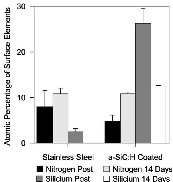
Figure 7. When the stents were left after the blood circulation experiment in platelet poor plasma, the nitrogen concentration further increased in both types of stents to a similar level. Simultaneously, the concentrations of chromium and silicon, as surface markers for the original material, reduced by half.
